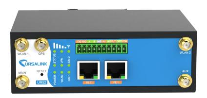
The Ursalink UR52 is a cost-effective industrial cellular router with embedded intelligent software features that are designed for multifarious M2M/IoT applications. Global WCDMA and 4G LTE carrier supported make this drop-in connectivity a great help for operators in maximizing uptime.
