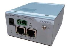
This IS-DG102S is equipped with 1 x 10/100/1000M TX PoE IN + 1 x 10/100/1000M TX for DATA OUT. It is capable to accept 60W PSE input to deliver 12VDC output (\*5V / 9V / 24V DC power output is also available). It can split power and data from PoE device. It is designed for environment where DC power source is not available. It can tolerate -40 to 75°C in harsh environment to perform a reliable network.
