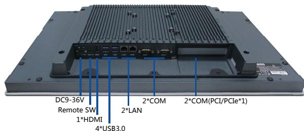
ALAD-K2120T(P) is an intelligent, fanless embedded panel, powered by Intel® Skylake-U/Kabylake-U Celeron or Core i3/i5/i7 CPU. ALAD-K2120T(P) supports 21.5 inches 1920\*1080@60Hz TFT LCD, with 1\*2.5 inch SATA HDD driver bay and 1\*M.2 for storage, DC 9~36V power input. It will be fit for application of MES and equipment management HMI terminal.
