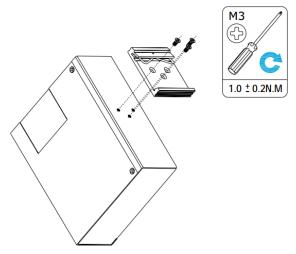
Use 3 pcs of M3\*6 flat head Phillips screws to fix the DIN rail to the router, and then hang the DIN rail on the mounting bracket. It is necessary to choose a standard bracket.
