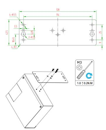
Use 3 pcs of M3\*4 flat head Phillips screws to fix the wall mounting kit to the router, and then use 2 pcs of M3 drywall screws to mount the router associated with the wall mounting kit on the wall.
