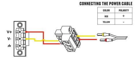
R3000 Router supports reverse polarity protection, but always refers to the figure above to connect the power adapter correctly. There are two cables associated with the power adapter. Following to the color of the head, connect the cable marked red to the positive pole through a terminal block, and connect the yellow one to the negative in the same way. The last step is to plug the power adapter into your socket.
