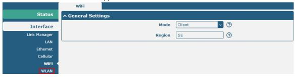
Click Interface > Link Manager > Link Settings, and click the edit button of WLAN, then configure the related parameters of WLAN.
