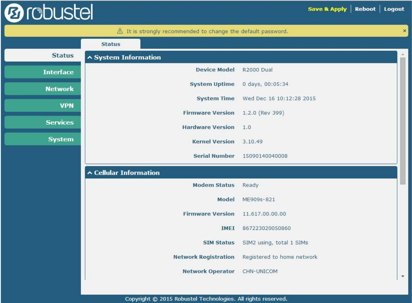
Using the original password to log in the router, the page will pop up the following tab
