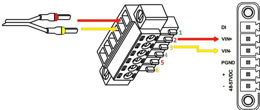
R2000 Dual Router also supports POE feature. Please refer to the figure below to connect the power adapter correctly.
