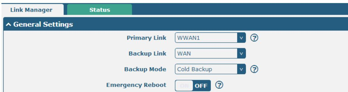
Link Settings section allows user to configure the parameter of link connection, include the WWAN1/WWAN2, WAN and WLAN. It is recommended to enable Ping detection to keep router always online. The Ping detection increases the reliability and also cost data traffic.
