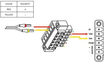
Step 7: R2000 Dual Router also supports POE feature. Please refer to the figure below to connect the power adapter correctly.
