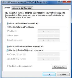
Manually configure the PC with a static IP address on the same subnet as the router address, click and configure "Use the following IP address";
