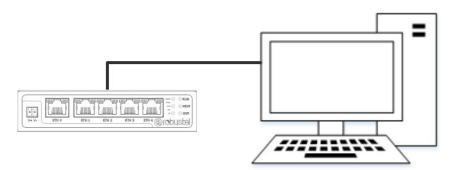
Connect the router's Ethernet port (ETH0~ETH4) to a PC with a standard Ethernet cable.
