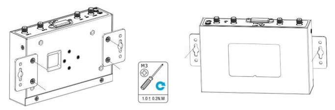
Use 4 pcs of M3 screws to fix the wall mounting kit to the router, and then use 2 pcs of M3 drywall screws to mount the router associated with the wall mounting kit on the wall.
