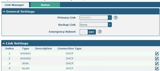
Click the button of WWAN1 to set its parameters according to the current ISP.
