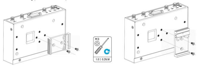
Use 2 pcs of M3 screws to fix the DIN rail to the router (as illustrations above shown, there are two mounting angles to choose from), and then hang the DIN rail on the mounting bracket.
