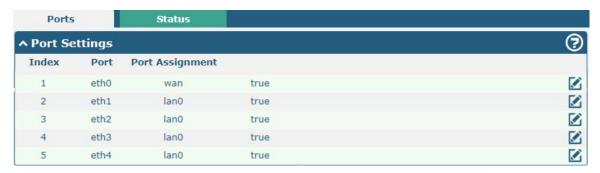
Click button of eth0 to configure its parameters, and modify the port assignment parameters of eth0 in the pop-up window.
