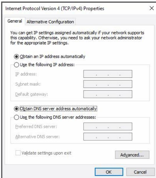
(2) Manually configure the PC with a static IP address on the same subnet as the device address, click and configure **"Use the following IP address"**;
