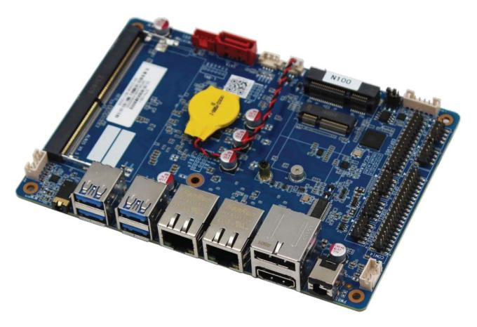
The 1ST-SBC-ALN35 is an embedded SBC board with the 12<sup>th</sup> Gen Intel® Processor N-series (Alder Lake-N) soldered on board.
