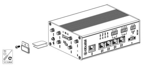
2. Antenna Installation. Rotate the antenna into the antenna connector accordingly.
