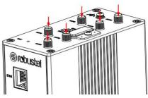
**3. Terminal Block Installation.** Insert the 3-PIN or 4-PIN terminal blocks into the interfaces connector, then can connect the devices or sensors to the router via corresponding interfaces.
